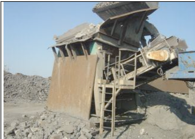
Installation de criblage.
